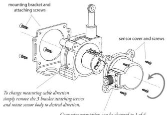
Connector orientation can be changed to 1 of 4 positions. Simply remove the 4 cover screws and rotate cover and replace screws.
