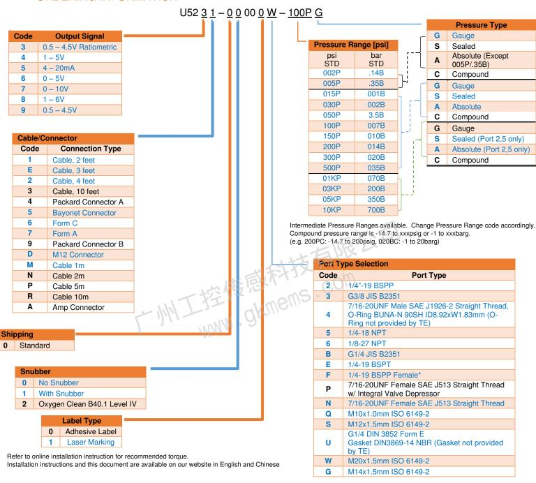
Standard In-Stock Models: M12 Connector, 1/4-18 NPT Pressure Port, Gage Type. These popular configurations below are typical units available off the shelf:
